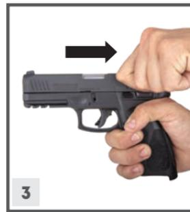
3. Hold the pistol with one hand keeping your finger away from the trigger and on the **memory pad**. With the other hand pull the **slide** to its limit and release it, the **slide** will go forward under **recoil spring** pressure and will insert one cartridge into the **chamber**.
