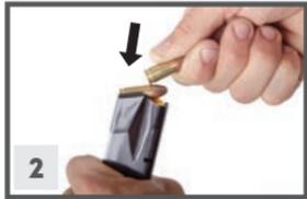
2. To load the **magazine** hold the bottom of the **magazine** with one of your hands and with the other one insert the cartridges one at a time, pressing them down and to the rear. Insert the **magazine** into the pistol until it is held by the **magazine catch**. If the **magazine** is not correctly inserted into the pistol, it can fall out when you intend to shoot.
