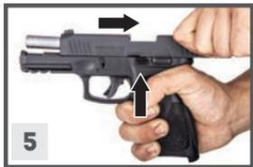
5. After the last round, the **slide** will remain in the open position held by the **slide catch**. In order to make it return to its rest position, press the **slide catch** downward just above the **left grip** or pull the **slide** to the rear and let the **slide** go forward (you must remove the empty **magazine** first).
