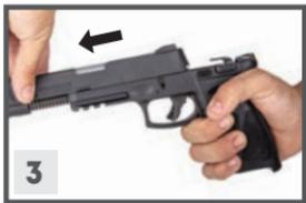
2. Hold the pistol in your hand in such a way that four fingers rest over the **slide** and your thumb rests on the rear of the **grip**. Using the fingers draw back the slide about 1/8". With your other hand, pull the **disassembly latch** down. Release the **slide**. Release **disassembly latch**.
