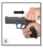
3. Hold the pistol with one hand keeping your finger away from the trigger and on the **memory pad**. With the other hand pull the **slide** to its limit and release it, the slide will go forward under recoil spring pressure and will insert one cartridge into the chamber.
