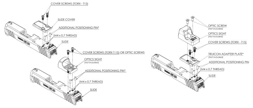
\*Additional positioning pins are only necessary for some models.
