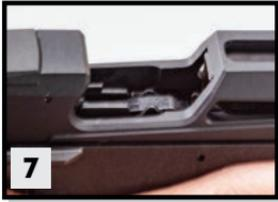
7. If you want to stop shooting before firing the last cartridge of a **magazine**, (1) keep your finger off of the **trigger**, (2) point the **muzzle** in a safe direction, (3) remove the **magazine** by pressing the **magazine release button**, (4) pull the **slide** to the rear and lock it back, and (5) look and feel the **magazine well** and **chamber** to confirm the pistol is empty. An empty firearm cannot fire.
