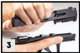
2. Hold the pistol in your hand in such a way that four fingers rest over the **slide** and your thumb rests on the rear of the **grip**. With the other hand, pull the **disassembly latch** down. Release the **disassembly latch**.
